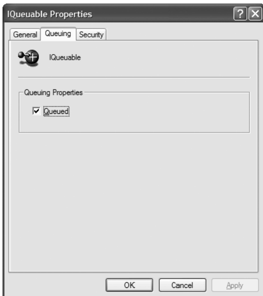
Figure 7-9. An interface configured for queuing
