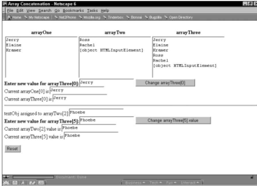
Figure 37-1: Object references remain “alive” in a concatenated array.
