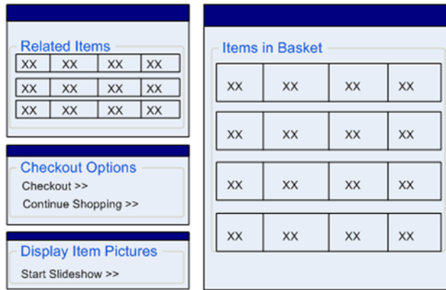
Figure 3.4 Breaking a large user interface down into smaller, individual components provides a way to reduce the complexity in a user interface.
