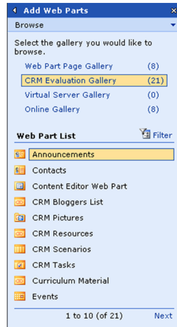
Figure 5.3 The CatalogZone in SharePoint provides elements for paging and filtering which cannot be achieved by simply specifying styles.
