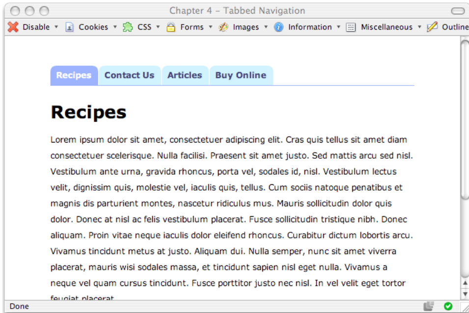
Figure 4.21. Highlighting the Contact Us tab by specifying contact as the ID of the body element
