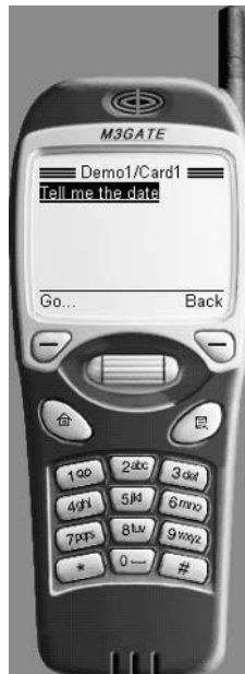
Figure 9.4 A WAP-phone emulator displaying the contents of a static WML page.
