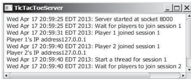
FIGURE 31.15 TicTacToeServer accepts connection requests and creates sessions to serve pairs of players.
