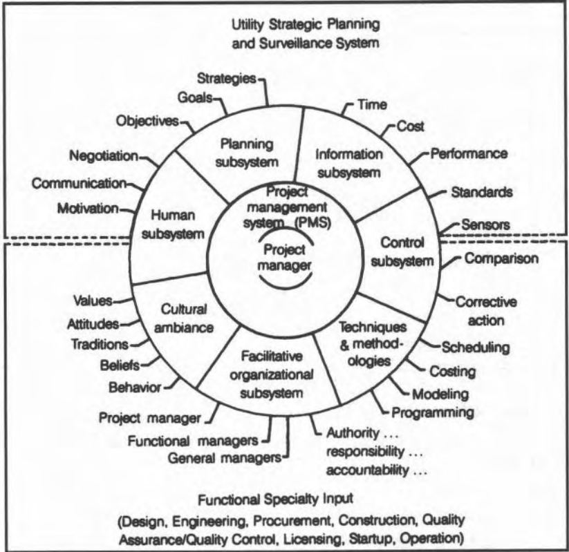
FIGURE 4.3 The project management system. (Source: Adapted from D. I. Cleland, "Defining a Project Management System," Project Management Quarterly , vol. 110, no. 4, p. 39.)
