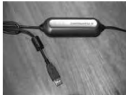
USB headphone/microphone combo and attached digitizing unit
