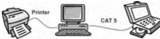
Simple network connecting two computers (via a CAT-5 cable) and a printer (via a printer cable).
