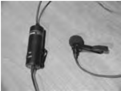
Line-in, powered, lavalier microphone
