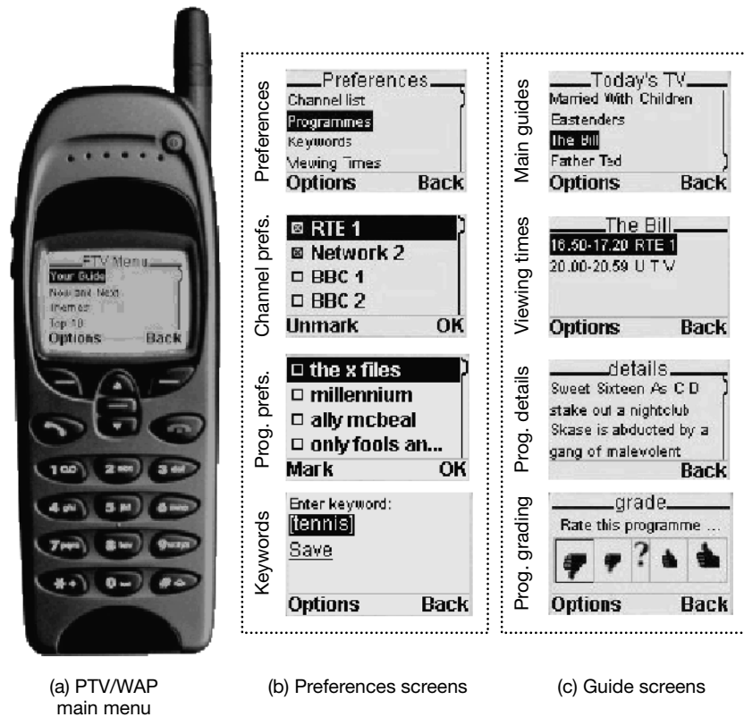
Figure 9.5 (a) The PTW/WAP main menu; (b) Preferences screens; (c) part of a personalized guide, including viewing times, program description, and grading screens.
